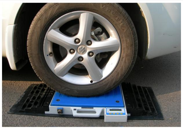
Truly portable, handy vehicle weighing system bringing vehicle weighment results at finger tips.
